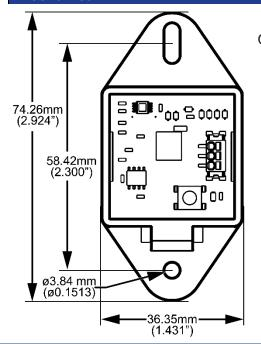
Submersion Depth 0.050" or 1.27mm Overall Dimensions 2.92" x 1.43" x 0.33"
